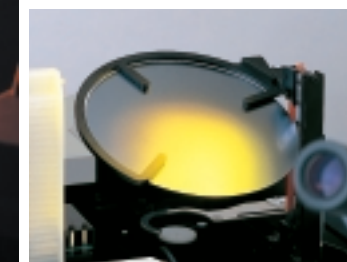
Back side center macro inspection (using a fiber optic illuminator)
